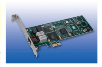
The entry-level offering is a low-profile one-span telephony board with software echo cancellation. The other Dialogic Blue Telephony Boards in the series have hardware echo cancellation and are available in one-, two-, four-, and eight-port versions with a half-length form factor. The entry-level board is suitable for installations of up to 2 ports, while the other boards scale to eight or more spans per system.
