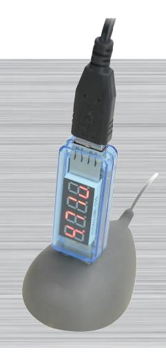
Measure the current consumption of any connected USB devices and display the consumption in volts and amps.
