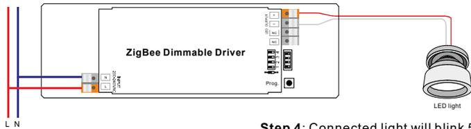
**Step 4:** Connected light will blink 5 times and then stay solid on, then the device will appear in your controller's menu and can be controlled through controller or hub interface.
