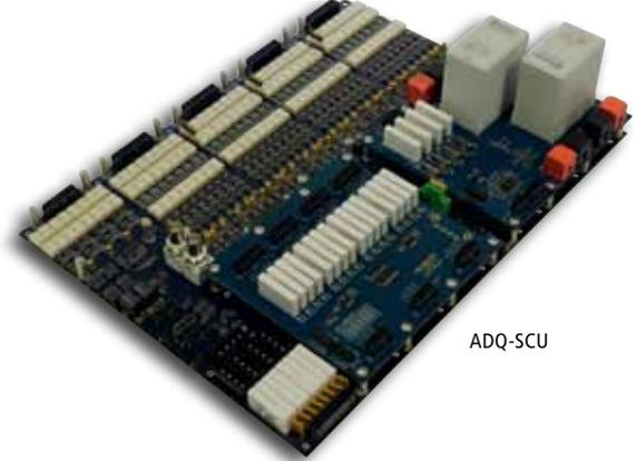
The ADQ-SCU signal conditioning unit was developed to optimally adapt a large number of analog and digital inputs/outputs to the requirements of a complex, automated test system. The signals are acquired and generated synchronously via the ADQ-344 multifunction measurement and control board, which also controls the ADQ-SCU via I<sup>2</sup>C bus.
