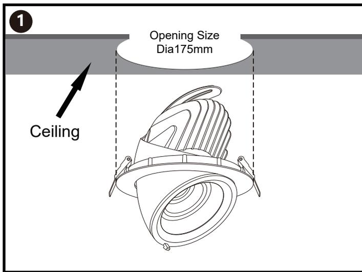
Prepare everything needed for installation & drill a hole with diameter 175mm in the ceiling.
