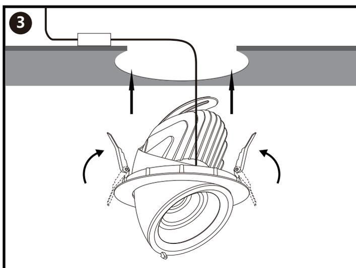
Pressing the springs while putting the lamp body into mounting hole.
