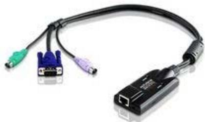
The KA7120 PS/2 KVM Adapter Cable connects the KVM switch and PS/2 mouse and keyboard ports of the target computer. With its form factor and light weight design, it represents the next generation KVM Adapter Cables – offering superior signal compensation and techniques for greatly enhanced video quality.
