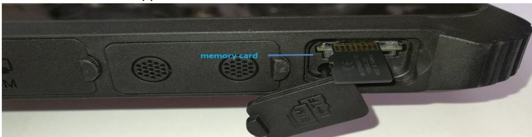
into the TF card slot as shown in the illustration (the SIM card slot is located above the TF card slot) Note: The metal side of the TF card faces the display.
