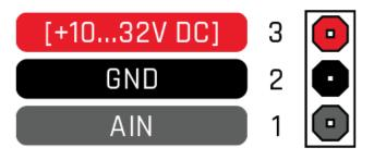
Figure 2 MSP500 socket pinout
