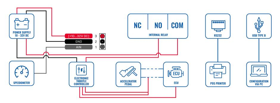
Figure 3 MSP500 Wiring scheme
