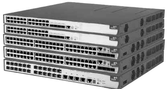
from top: 3Com Switch 5500G-EI 24-Port, Switch 5500G-EI PWR 24-Port, Switch 5500G-EI 48-Port, Switch 5500G-EI PWR 48-Port, Switch 5500G-EI 24-Port SFP
