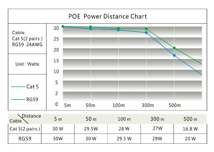
Notes: In the above figure, the left vertical coordinate is the PoE output power, the bottom horizontal coordinate is the PoE transmission distance, please compare the horizontal and vertical coordinates at the same time to get the exact corresponding output power.
